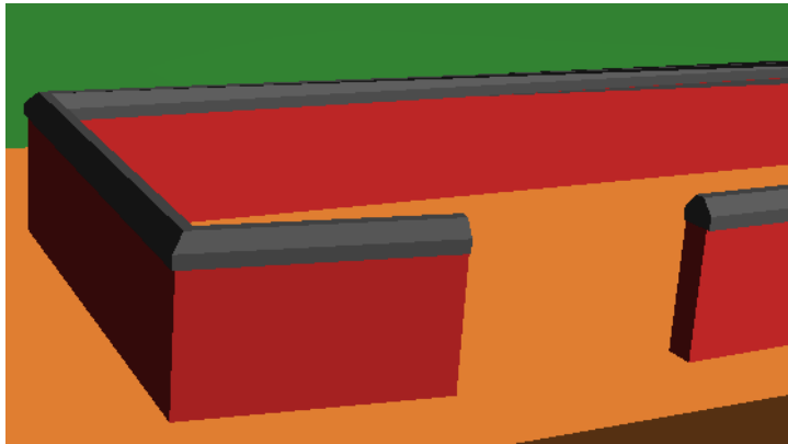
Figure 80: Wall with coping stones
